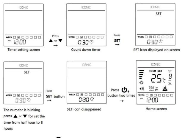
Press the clock button O when home screen, 1 icon displayed on the screen, the weekly schedule 1 will be enabled, press again clock button, 2 icon displayed on the screen, the weekly schedule 2 will be enabled. Press again clock button the C icon on displayed on the screen, the countdown timer is enabled. If no 1 or 2 and C displayed on the screen, the weekly timer schedule and countdown timer will be disabled
